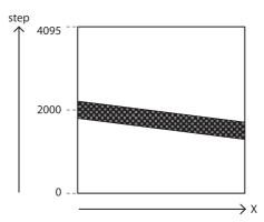
Execute opaque defect point detection. Like the clear defect point detection, set the image pickup conditions and the threshold in units of 14 bits. Below is an example for 10000 step/14bit. Pixels that indicate 0 to 10000 steps are detected. If are not setting opaque defect points, you can skip this step.
