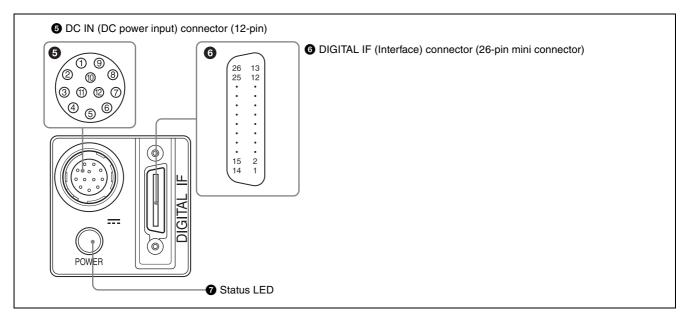
**OC IN (DC power input) connector (12-pin)** You can connect a camera cable CCXC-12P05N etc. to input the 12 V DC power supply. The pin configuration of this connector is as follows. You can operate the camera without using this connector when using a PoCL-compatible camera module interface board. For details on the pin arrangement, see the following table.
