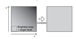
**2** Adjust the exposure and other parameters so that the target level is about 50%. On color cameras, adjust the white balance.
