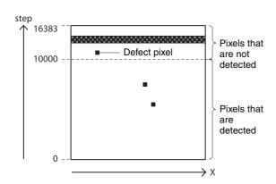
5 Select the data for applying defect correction. To apply the pixels detected in steps 3 and 4, select 2. To apply factory settings, select 0. To apply values that have been saved, select 1. >DEFECT-PATTERN-LOAD 2
