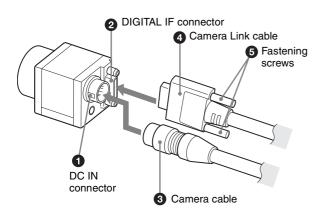
Connect the camera cable to the DC IN connector and the Camera Link cable to the DIGITAL IF cable respectively. If you use a camera module interface board with support for PoCL, you can operate the camera even if you do not connect the camera cable to the DC IN connector. When you connect the Camera Link cable, turn the two fastening screws on the connector to secure the cable tightly.
