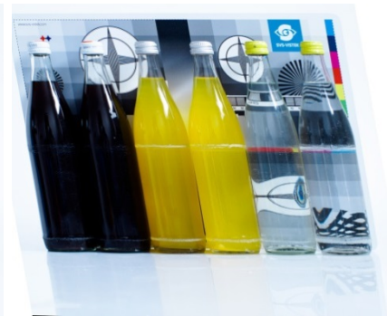
Figure 10 rolling shutter with moving objects(geometric distortion)
