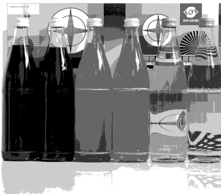
Figure 19: Figure of quantification with 6 shades of gray (reduced colour depth)
