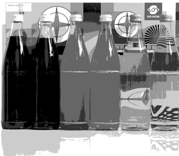
Figure 25: Figure of quantification with 6 shades of gray (reduced colour depth)
