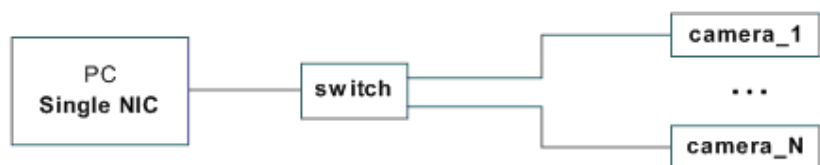
FIGURE 10: ILLUSTRATION OF CONNECTING MULTIPLE CAMERAS WITH A SWITCH
