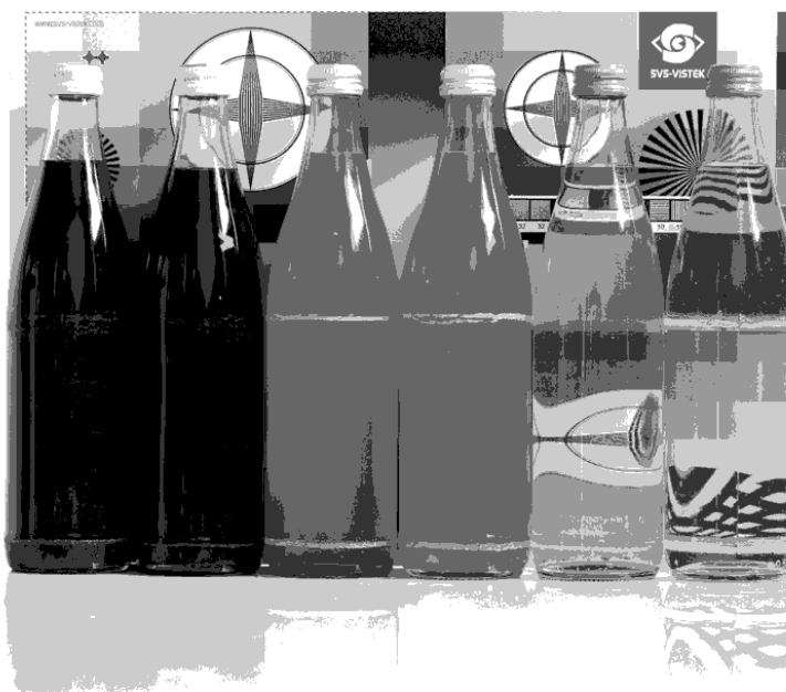
Figure 22: Figure of quantification with 6 shades of gray (reduced colour depth)
