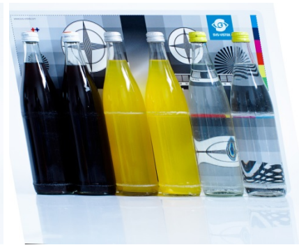
Figure 15 rolling shutter with moving objects (geometric distortion)
