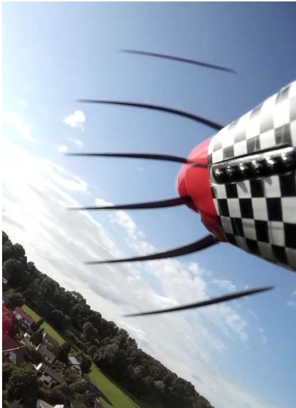
Figure 13: Rolling shutter with fast moving object details
