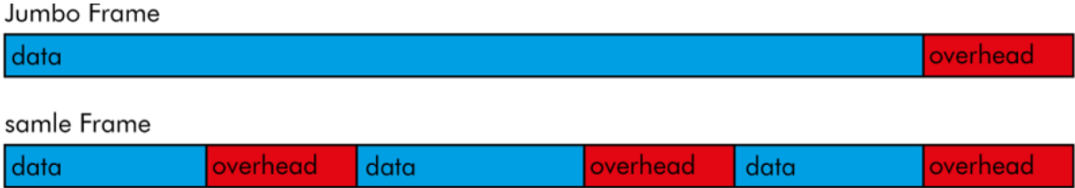
FIGURE 8: ILLUSTRATION OF DATA REDUCTION WITH JUMBO FRAMES
