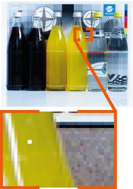
Figure 63: Illustration of a defect pixel
