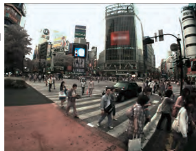
Standard wide angle lens f=3.3mm (horizontal angle 104.3°)
