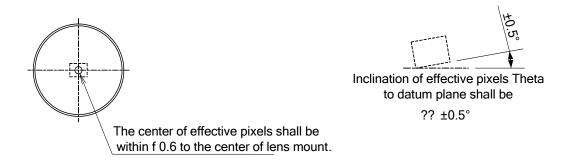
(\*) Dimension from datum plane to the center of lens mount.
