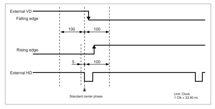
Make sure that the external HD and VD phases against the standard center phase are as shown in the figure.
