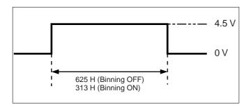
The amplitude level is the typical value when terminated with 10 k  $\Omega.$
