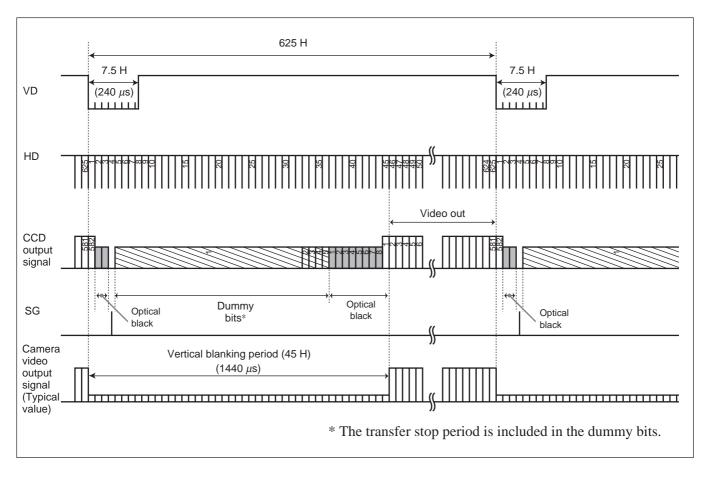
Vertical Output Waveform Timing Chart (Binning ON)
