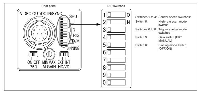
\* The electronic shutter cannot be used in restart/reset mode. High-rate scan can be used in restart/reset mode and in external trigger shutter mode 1.
