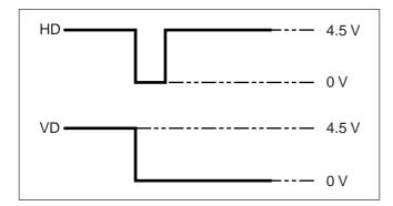
The amplitude level is the typical value when terminated with 10 k $\Omega$ . External HD and VD can be output when you set the HD/VD signal input/output switch to INT.
