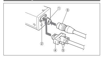
Connect the camera cable to the DC IN connector and the LAN cable to the RJ45 connector respectively. When you connect the LAN cable, turn the two fastening screws on the connector to secure the cable tightly.
